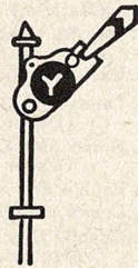
Fig. 137A Rule 285 Indication: Prepare to stop at next signal. Train exceeding medium speed must at once reduce to that speed. Name: Approach.
